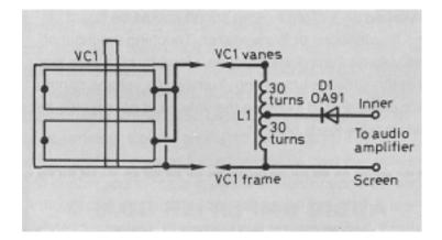
Figure 1 Both sets of moving vanes are joined as shown. L1 is wound on a ferrite rod with 32 SWG wire and centre-tapped. A single winding (no tap) can be used, joining D1 to the top of the winding
